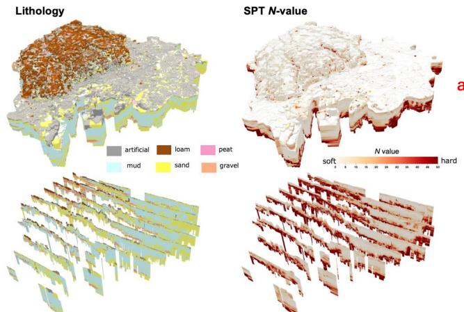
These **soft muddy sediments** have a potential risk of **amplifying earthquake ground motion**.
